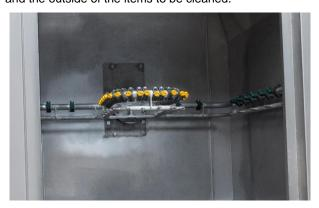
This rotating spraying pattern is motor-actuated and is mounted on the back of the cabin washer. Additionally the loading door is equipped with a built-in fixed or rotating spraying pattern to clean the outside bottom of the items to be washed.
