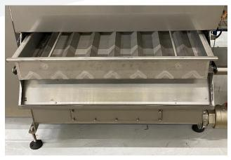
The Cretel cabin washer is standard equipped with a static filter which is manually removable for cleaning purposes. The design is made to create a maximum filtering capacity even in case of intensive soiling.
